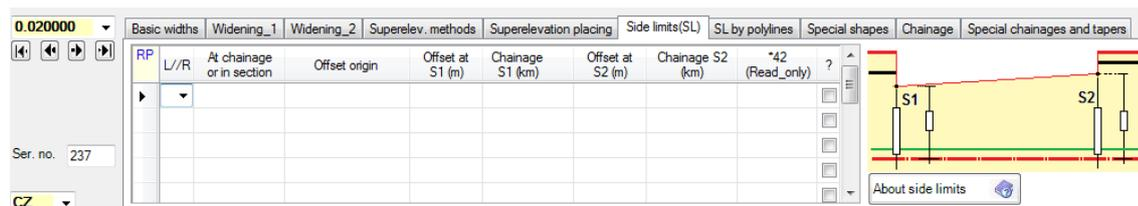
Table placed on tab **SIDE LIMITS (SL)** enable to assign side limits borders for numerous of cross sections given in segment or for individual cross section. The assigned segments can follow each other but cannot layover. Inside of the segment an individual cross section can be assigned. In that case will be not used interpolated value from segment but the value of side limits for individual cross section is respected.
